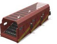
Long-lasting steel discs provide lateral agitation to separate large cardboard from other fibers. containers, and debris.
