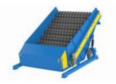
Performs 2D/3D separation and is especially designed to reduce wrapping.
