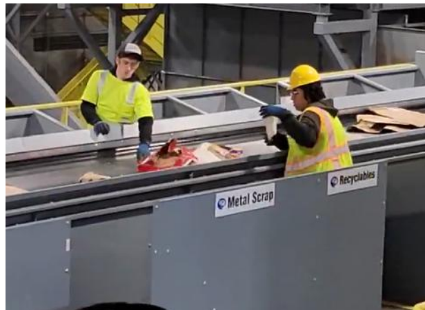
The new, innovative MRF design. Decreased material burden depth, less sorters needed, and improved worker safety. The machine is before any sorters.
