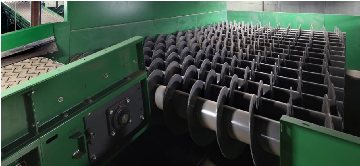
Primary Auger Screen (Cal-Waste Galt, CA). Three sorters on screen post-sort. No sorters prior to screen.
