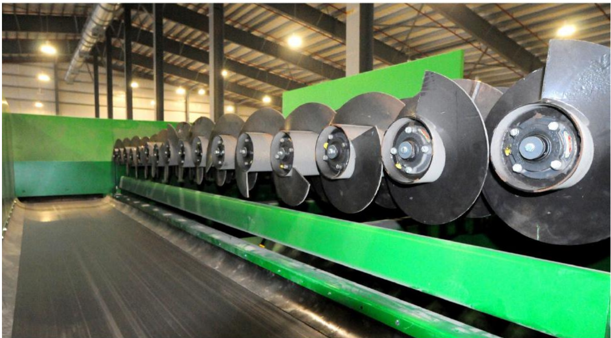
An auger screen goes directly after the infeed conveyor at a MRF and needs no presorting.
