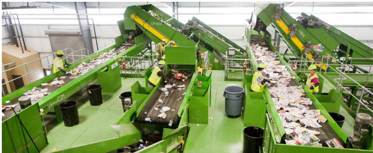
2012 MRF – a decade plus ago, finished products were largely produced directly from the fractions of disc screens, with some manual Q C. Modern MRFs require more separation automation due to the significant changes in the material stream.
