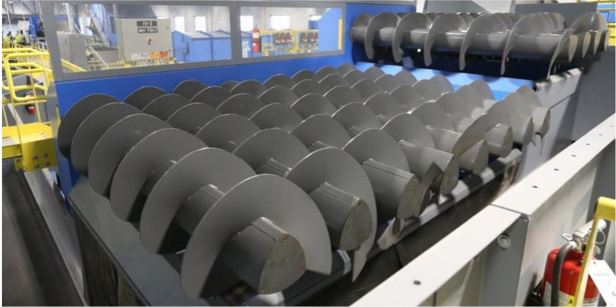
OCC Auger Screen (MWA, Des Moines, IA). Two to three OCC QC on screen post-sort. No manual sorters prior to screen.
