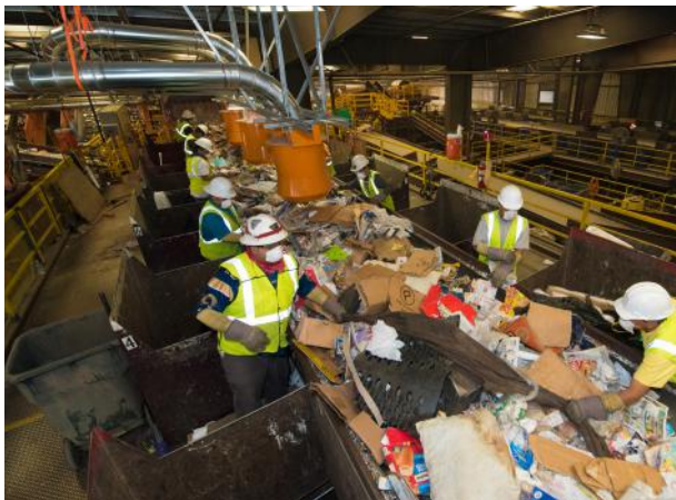
The old way of designing an MRF. Overburdened, high material depth, unsafe workspace, many sorters needed and a typical system bottleneck. No machines before the sorters.
