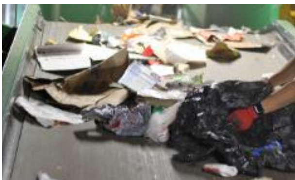
The fraction that goes over the Auger Screen. The manual post-sort station only sees large material with a significantly reduced burden depth.
