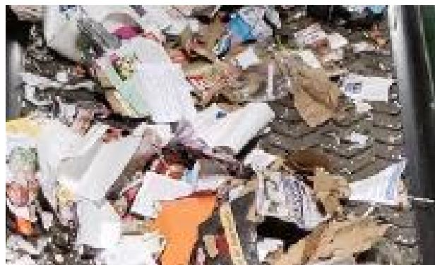
The fraction that falls through the Auger Screen - 60% of material, including sharps or other unsafe material, bypasses all manual sorters.
