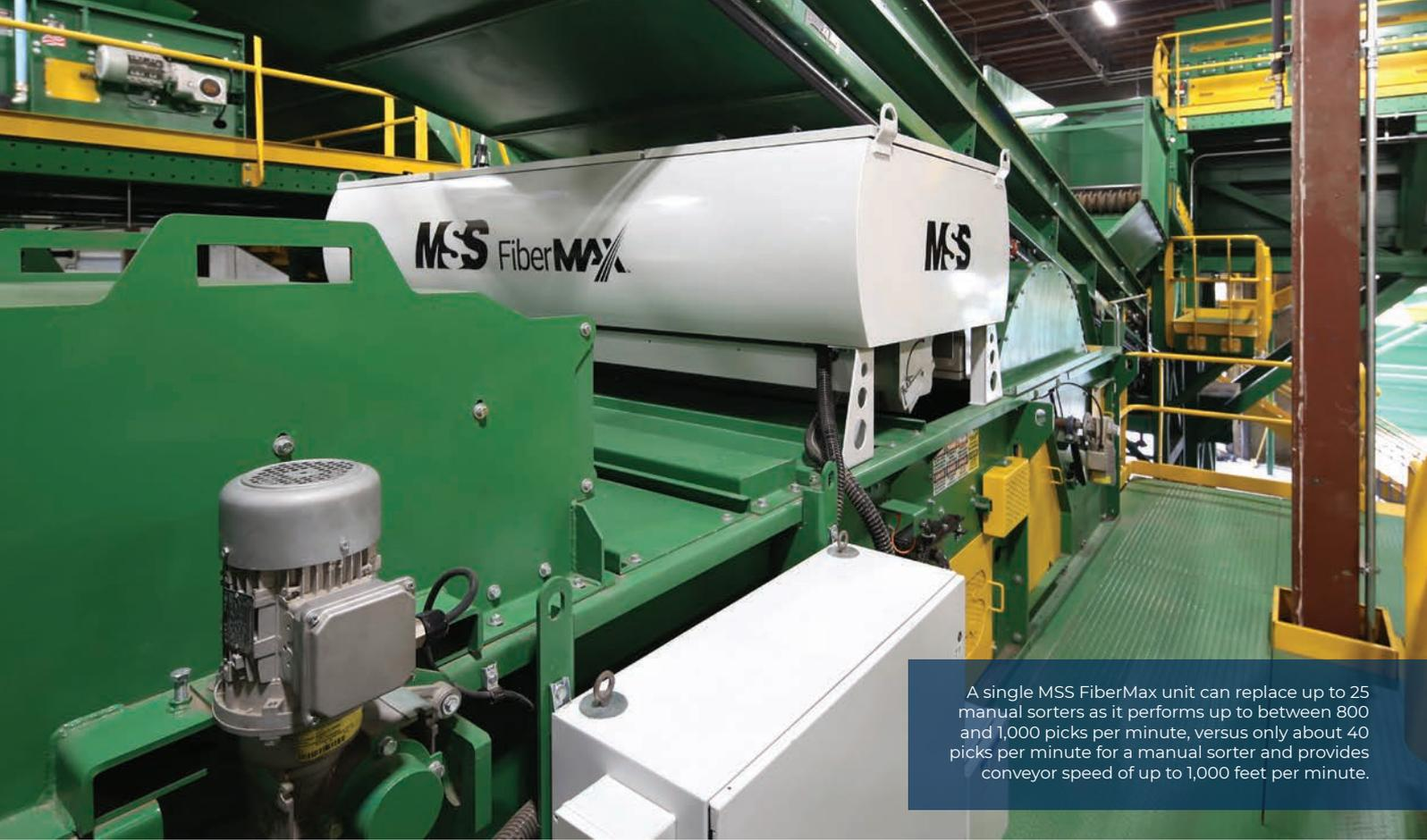
A single MSS FiberMax unit can replace up to 25 manual sorters as it performs up to between 800 and 1,000 picks per minute, versus only about 40 picks per minute for a manual sorter and provides conveyor speed of up to 1,000 feet per minute.
