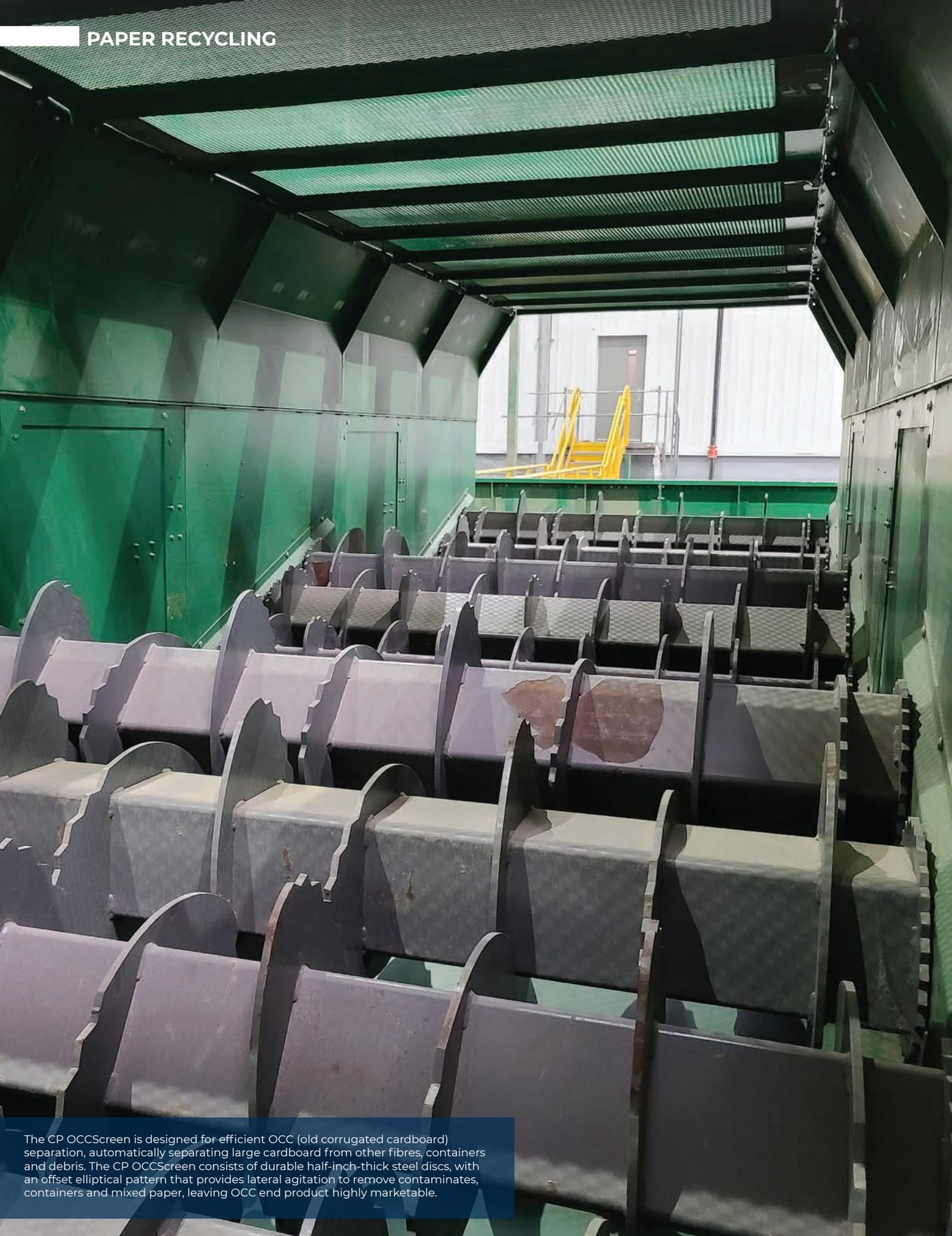
The CP OCCScreen is designed for efficient OCC (old corrugated cardboard) separation, automatically separating large cardboard from other fibres, containers and debris. The CP OCCScreen consists of durable half-inch-thick steel discs, with an offset elliptical pattern that provides lateral agitation to remove contaminants, containers and mixed paper, leaving OCC end product highly marketable.
